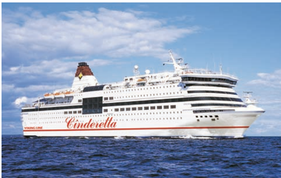
By fitting SCR to all its engines, the emissions of nitrogen oxides from Viking Line's MS Cinderella are cut by 97%, down to 0.4 g/kWh. MS Cinderella also uses low-sulphur (< 0.5%) fuel, and is in Stockholm connected to shore-side power.
